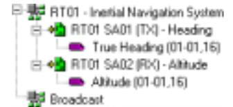
them to the hardware tree. Users may enable or disable transmit and receive SAs, configure/legalize mode codes, and create a unique status mask for each RT. Complete RT profiles can be saved to and loaded from the 1553 database.
