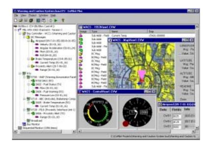
With CoPilot 1553 Plus, users can view and edit data through strip charts, moving map displays, and virtual controls. Plus users can analyze with software playback, test with hardware playback, or customize CoPilot with scripting.
